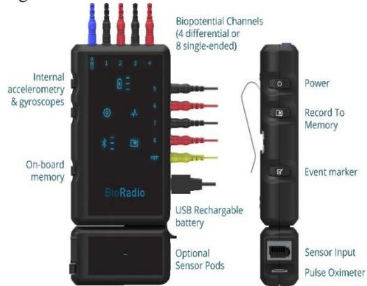
Figure. 5 BioRadio Technology[13]
